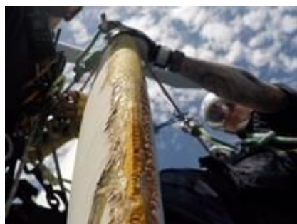
Figure 6: Leading edge erosion
